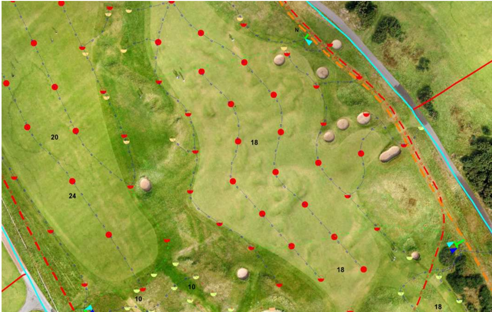
Old Course St Andrews – 5 th Fairway 'after', sprinklers at 18m triangle spacing – multi
